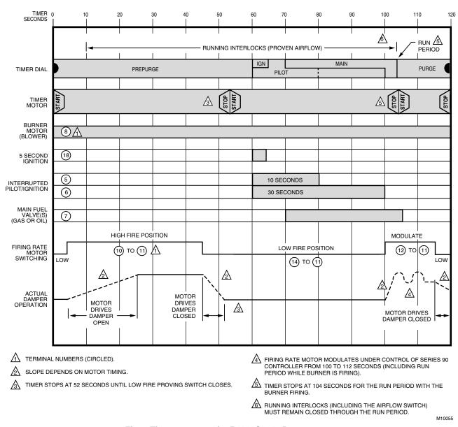
Fig. 8. Timer sequence for R4140G1049 Programmer.
